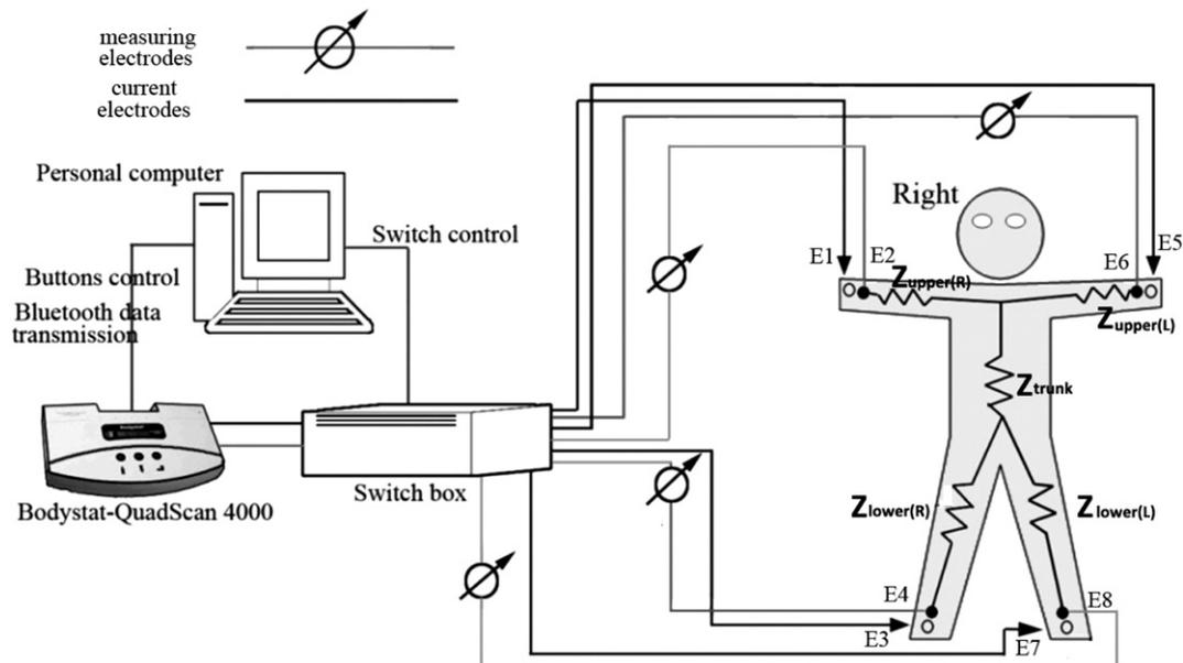
**Fig. 1.** The modified BIA instrument with eight electrodes ( $BIA_8$ ). With a circuit between E1 and E3, measurement between E2 and E4 yields  $Z_{whole}$ , measurement between E2 and E6 yields  $Z_{upper(R)}$ , measurement between E2 and E6 yields  $Z_{upper(L)}$ , measurement between E4 and E8 yields  $Z_{trunk}$ . With a circuit between E5 and E7, measurement between E4 and E8 yields  $Z_{lower(L)}$  and measurement between E2 and E6 yields  $Z_{upper(R)} + Z_{lower(R)} + Z_{trunk}$ .
